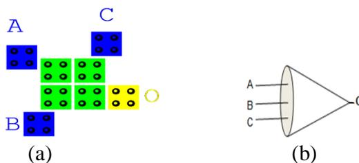
Figure 4: FNZ Gate (a) QCA Design, and (b) Symbol
