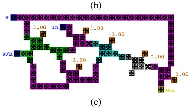
Figure 3: The RAM cell structure (a) schematic diagram, (b) FNZ based QCA Implementation, and (c) FNZ based QCA Implementation with reduced cell count.
