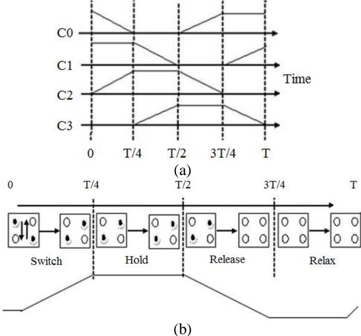
Figure2. QCA clocking: (a) Four-phase (b) working procedure during one clock phase
