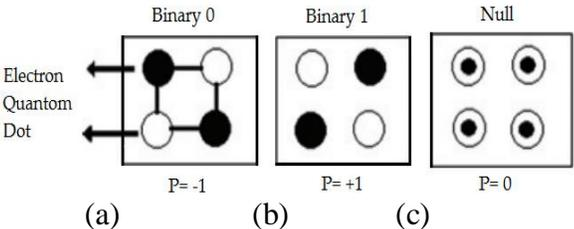
Figure1. Different QCA cell polarizations
