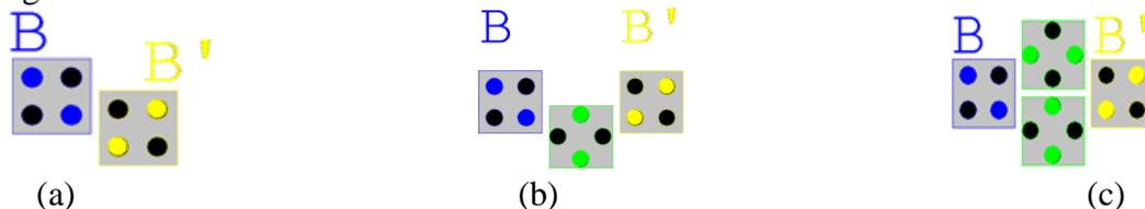
Figure3. QCA implementation of Inverters
